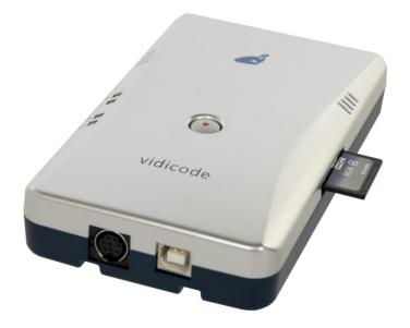
The V-Tap ISDN PRI is a device that can record the calls from an ISDN-30 E1 line.
