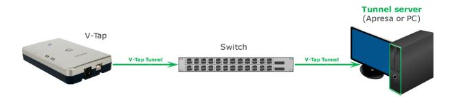
A connection between the V-Tap and the V-Archive PC software (or Apresa recorder) is needed to get the recorded data automatically into a user accessible database.
