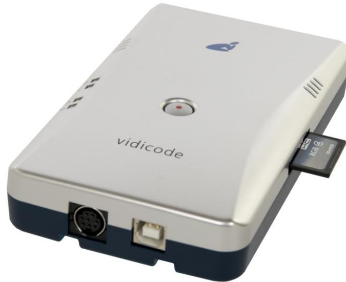
The V-Tap Analog is a device that can record the audio from an analog telephone line or any telephone that works with a handset. The recorded calls are stored onto an SD card and can optionally be sent to an external server, which can be a [Call Recorder Apresa](#) or the [V-Archive software](#) running on a PC.
