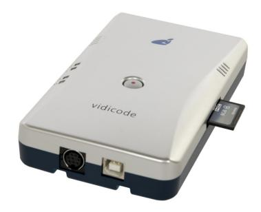
The V-Tap Analog 2 is a device that can record the audio from an analog telephone line or any telephone that works with a handset. Additionally, there is a 3.5 mm stereo input jack that enables recording from other audio sources, such as microphones or radio's. The recorded calls are stored onto an SD card and can optionally be sent to an external server, which can be a <u>Call Recorder Apresa</u> or the <u>V-Archive software</u> running on a PC.
