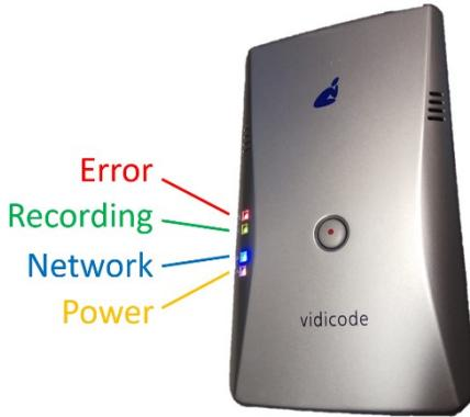
**Red LED steady on:** To indicate an error. If the Red LED is on, the device is not booting or an SD card is not detected.
