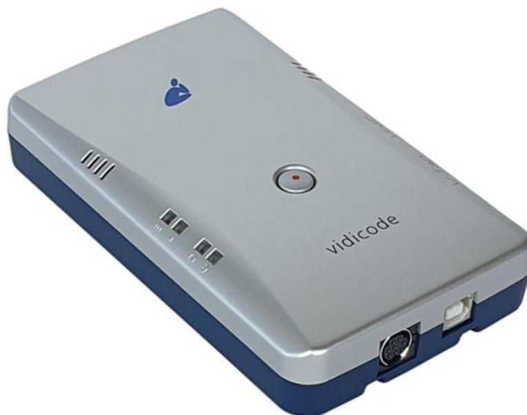
The V-Mic is a hardware and software solution for the recording of audio, coming from a microphone. The supplied hardware unit can operate stand-alone and has a built-in microphone, but can also be connected to a professional external microphone. The recorded data is stored onto an SD card and can optionally be sent to an external server, which can be a [Call Recorder Apresa](#) or the [V-Archive software](#) running on a PC.
