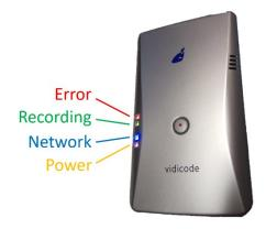
**Red LED steady on:** To indicate an error. If the Red LED is on, the device is not booting or an SD card is not detected.
