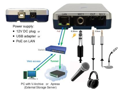
To fine-tune the audio settings or to setup a connection to external software, you have to access the settings in the web interface. Then it is needed to connect with the network, using a browser (see here).
