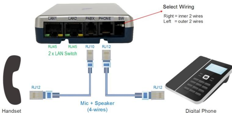
The position of the Wire-select-switch can be to the left or to the right, depending on the wiring inside the handset-cable.
