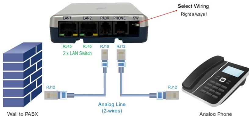
The position of the Wire-select-switch is always to the right in this case.
