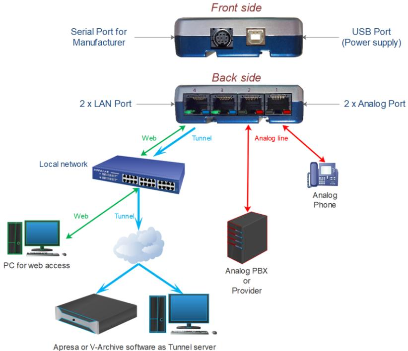
Two possible ways to connect the V-Tap Analog (line and handset) are shown in the next two schemes.
