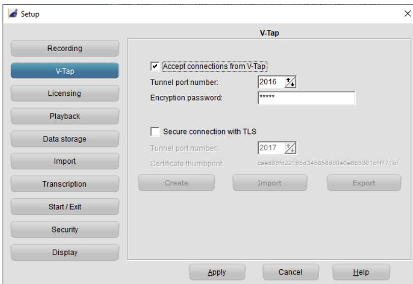
**NOTE1:** The PC's IP address is the "Tunnel Server Address" in the V-Tap.
