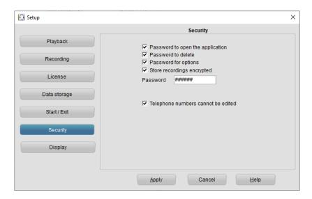
It is possible to protect the Oygo application with a **password**. Deleting of recordings and settings of the program can be protected separately.
